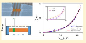
width of the  $Ga_xIn_{1-x}Sb$  tunnel barrier are extracted from the Wentzel-Kramers-Brillouin (WKB) fits to the experimental I-V traces.
